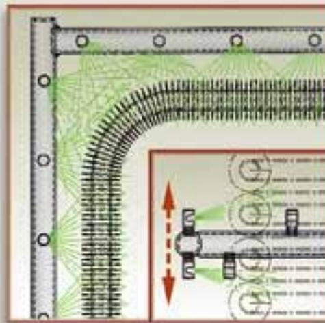
Proper sootblowing is necessary when fuel has a high sulphur content or combustion is poor (such as No. 6 fuel oil). Without sootblowing, the finned tubing will become fouled and the maximum heat recovery cannot be achieved.
