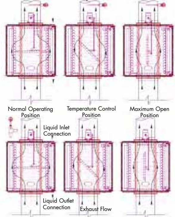
Liquid Temperature Control Assembly (above)
